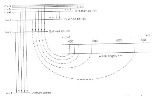
Electron transitions to the n = 2 level occur in the visible region and correspond to the Balmer Series. Transitions to the n = 1 level release more energy; lines appear at higher frequencies in the UV region and correspond to the Lyman Series.
