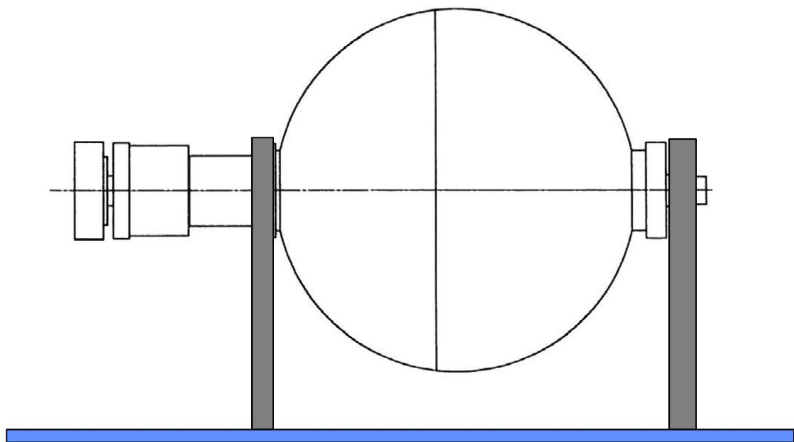
The motors are as shown, below, also secured to the base plate. And for example, a 22mm slide motor may be an aluminum block with a sliding bore 22 is used on one side that is slit, at right angles to this slitvlak is a bolt which clamps the engine. Any strap length adjustments by lateral displacement of the block (slit in the base plate or shim between base plate and motor unit)
