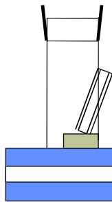
The mounting of the main bearings is best done in bearing blocks which in turn are on a base plate. These main bearings have bars with a bore for the bearing arrangement and positioning with circlips which are after assembly then bolted to the bottom plate, but there is a slightly more expensive but more elegant method wherein the bearing mount has been split in a support with a lid (cap), wherein the whole in the bearing arrangements can be made and then attached with the caps
