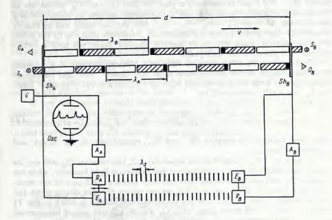
Figure 1. The ultrasonic "coupled-shutters" experiment.
