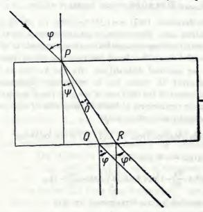
Figure 3. The drag aberration.
