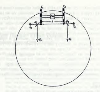
Fig. 8. Coupled shutters mounted on a rotating disk for d much less than  $2\pi R$ .
