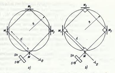
Fig. 2. The rotating disk experiment: (a) The Harress-Marinov variant, (b) the Harress-Dufour variant.
