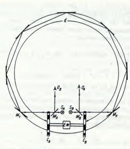
Fig. 7. Coupled shutters mounted on a rotating disk for d near  $2\pi R$ .
