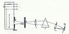
Fig. 1. Scheme of the experiment for the establishment of the zero transverse light Doppler effect.
