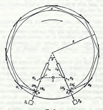
Fig. 2 The "coherent lasers on a rotating disk" experiment.
