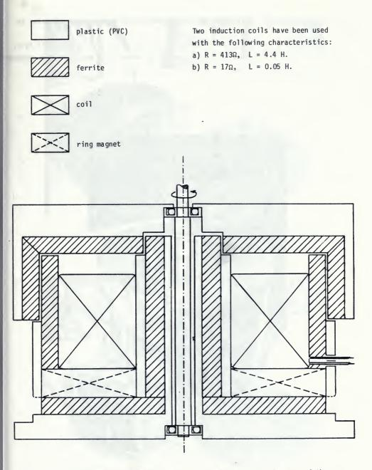
Fig. 17. - Diagram of the second VENETIC COLIU machine. The diameter of the rotor is 18 cm.
