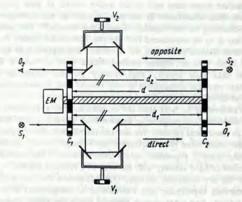
Fig. 5. Rigidly connected coupled shutters.
