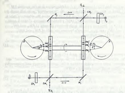
Fig. 1. The interferometric "coupled-mirrors" experiment.
