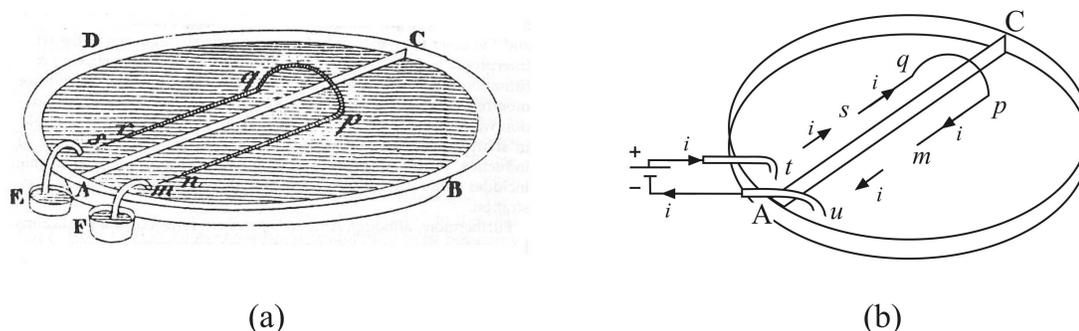
Figure 8.3: (a) Ampère's bridge experiment. (b) Our illustration indicating the directions of the current. The bridge is represented by the segment  $sqpm$ .
