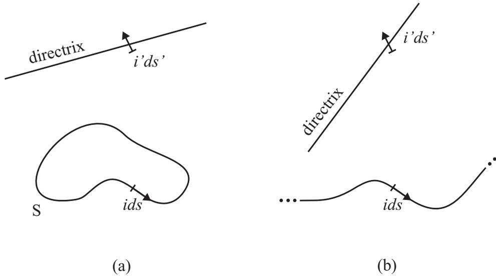
Figure 10.1: (a) Directrix due to a closed circuit of arbitrary shape passing through the center of the current element  $i'ds'$  located at an arbitrary point in space. (b) Directrix passing through the center of  $i'ds'$ , due to a circuit of arbitrary shape extending indefinitely in both directions.
