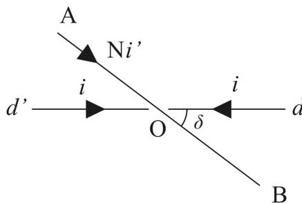
Figure 4.22: Upper view of figure 4.21 indicating only the lower portions  $d'e'$  and  $de$  of the astatic coil, together with the upper horizontal portion  $AB$  of the rectangular coil below the astatic coil.
