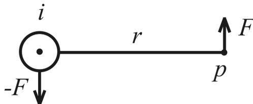
Figure 13.1: A long straight wire normal to the plane of the paper, with a current  $i$  coming out of the paper. The arrows indicate the forces exerted between a North pole  $p$  of the magnetized needle and the current-carrying wire, according to Faraday's conceptions.
