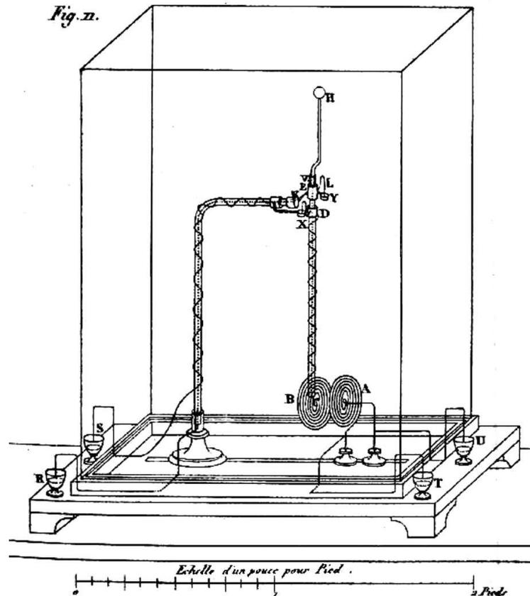
Figure 3.8: Ampère's first observation of attraction and repulsion between two current-carrying conductors. Spiral *A* remains fixed in the laboratory, while spiral *B* is mobile in such a way that it can move towards spiral *A* or away from it.
