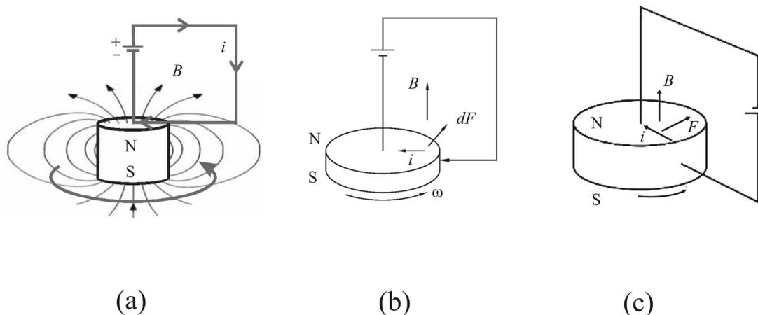
Figure 21.11: Modern explanations for the rotation of a magnet around its axis utilizing his own magnetic field  $B$  and the force exerted by this magnetic field acting on a current flowing inside the magnet.
