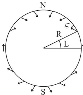
Figure 10.23: Dip angle  $\zeta$  as a function of the latitude angle  $L$ . The letter  $R$  indicates the Earth's radius.
