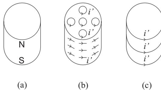
Figure 16.3: (a) Cylindrical magnet. (b) Ampère's molecular currents of intensity  $i'$ . (c) Effective electric currents flowing on the surface of the magnet due to the cancellation of the microscopic currents in any internal point of the magnet.
