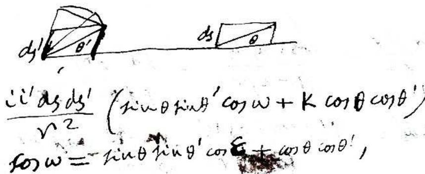
Figure 2.21: Ampère's drawing representing the angles  $\theta$  and  $\theta'$ .
