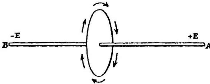
Figure 11.3: Ørsted's figure representing the magnetic action of a straight current-carrying conductor.
