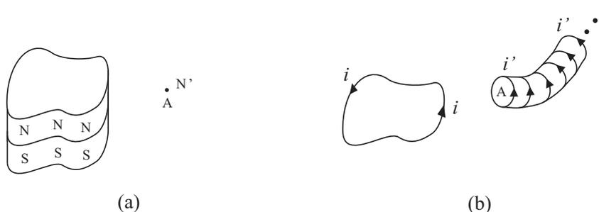
Figure 10.25: (a) Magnetic surface composed of a magnetic dipole layer interacting with a magnetic pole  $N'$  located at point  $A$ . (b) Current carrying closed circuit following the contour of the magnetic surface and interacting with a simply indefinite solenoid with its extremity located at point  $A$ . The forces acting on these two configurations, (a) and (b), have the same behavior as regards the angles and distances involved in these problems.
