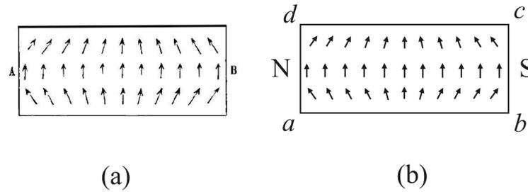
Figure 5.6: Ampère's improved conception of the molecular currents for a cylindrical magnet.
