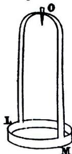
Figure 7.5: Mobile conductor of the instrument of figure 7.4.
