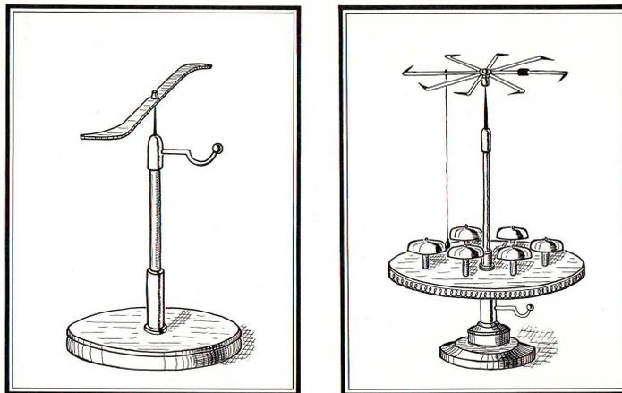
The apparatus normally turns around a vertical axis when connected to a source of high tension. It works based on the so-called electric wind and does not rotate in vacuum. There is a long controversy related to its working mechanism, [Robinson, 1962].
