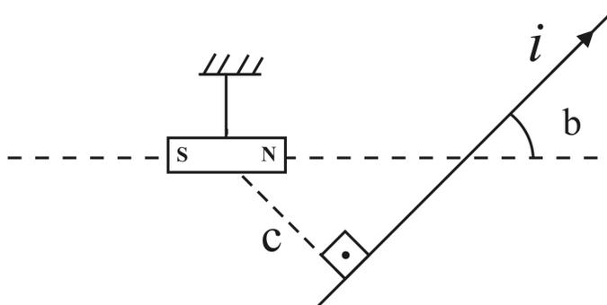
Figure 6.7: A long straight wire located in the vertical plane of the paper, making an angle  $b$  with the horizontal. A small horizontal magnetized needle has its center at a distance  $c$  to the wire.
