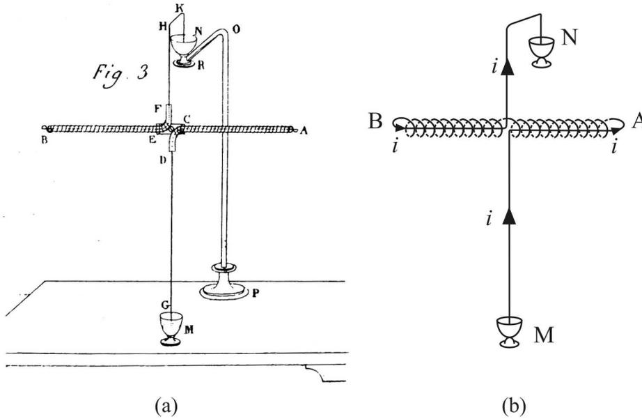
Figure 3.11: (a) Ampère's helix. (b) Our reproduction of this figure indicating the current sense in this experiment.
