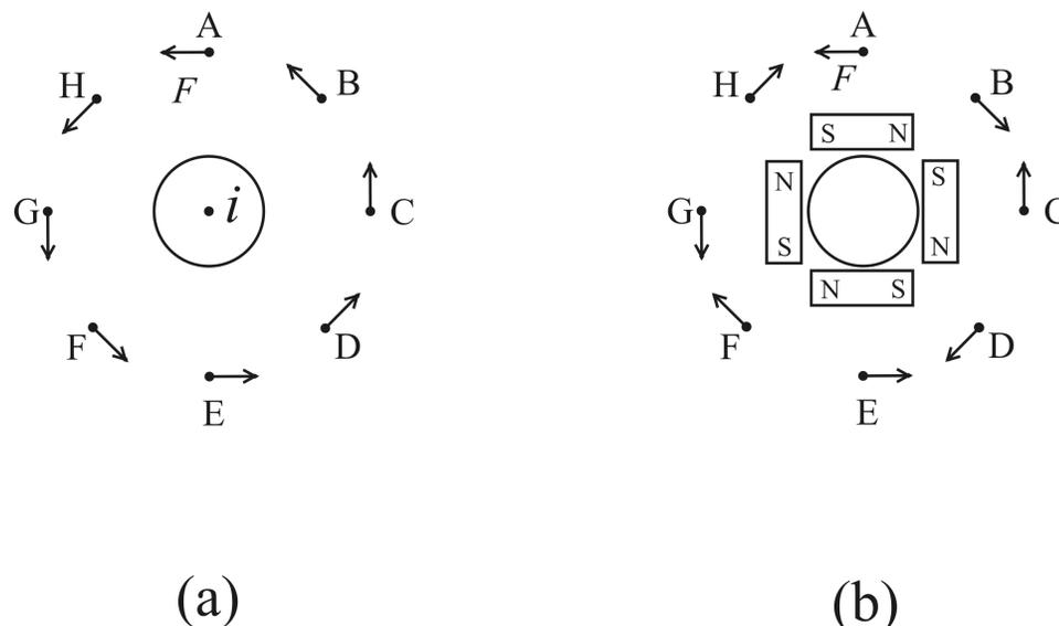
Figure 18.3: (a) Directions of the force acting on a North pole placed around a current-carrying wire according to Ørsted's experiment. (b) Directions of the force acting on a North pole placed around a current-carrying wire according to the magnetization of this wire as suggested by Biot and Savart.
