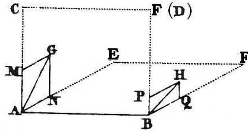
Figure 4.11: Ampère's figure with which it is possible to illustrate the addition law in the particular case of the interaction between the current elements  $AG$  and  $BH$  which are orthogonal to the straight line  $AB$  connecting their midpoints. The plane  $BACF(D)$  is orthogonal to the plane  $BAEF$ .
