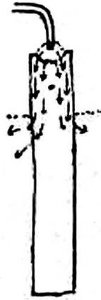
Figure 21.6: Faraday's illustration of the electric currents flowing inside the magnet. The central dot represents the magnetic pole while the arrows indicate the directions of the electric currents.
