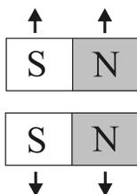
Figure 4.6: Two bar magnets repelling one another.
