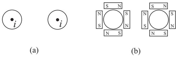
Figure 21.2: (a) Two straight wires carrying currents in the same direction and attracting one another. (b) Biot and Savart's explanation of this effect supposing the magnetization of both wires and the interaction of the supposed magnets distributed around the cross sections of both wires.
