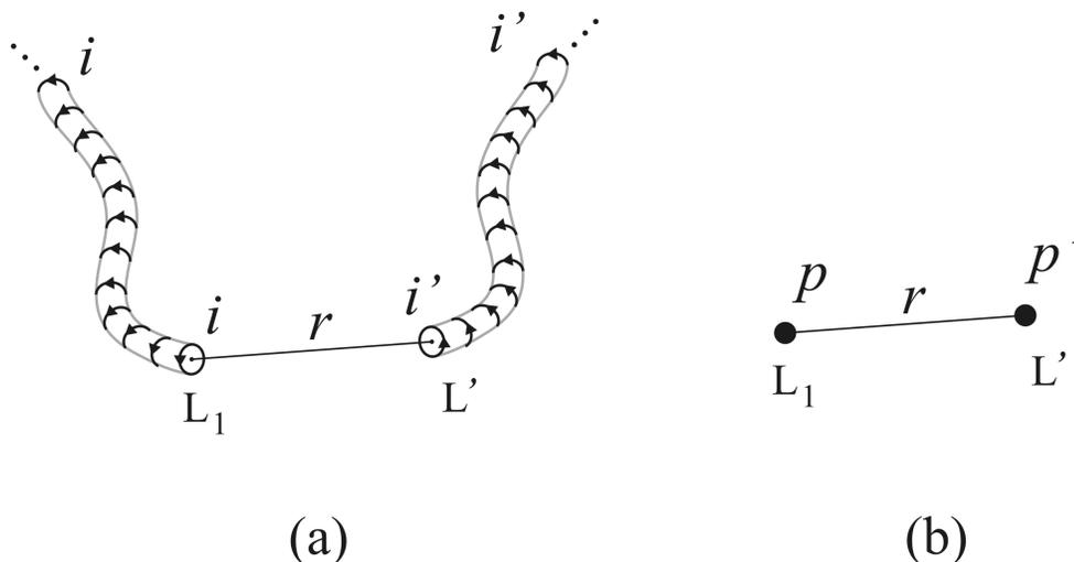
Figure 10.9: (a) Two simply indefinite solenoids with the centers of the extremities located at points  $L_1$  and  $L'$ , separated by a distance  $r$ . (b) Magnetic poles  $p$  and  $p'$ , separated by a distance  $r$  and located at points  $L_1$  and  $L'$ .
