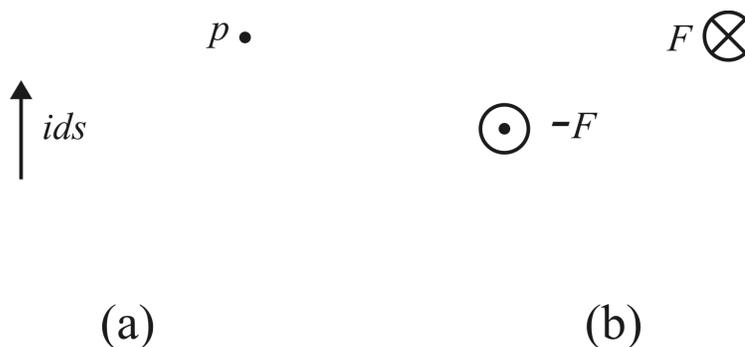
Figure 20.4: Primitive couple according to Biot and Savart's law.
