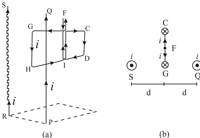
Figure 4.18: (a) Schematic representation of the direction of the current in the experiment of figure 4.17. (b) Case of equilibrium of the sinuous wire seen from above.
