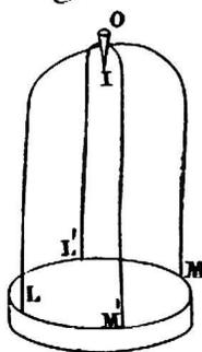
Figure 7.6: With this instrument Ampère obtained a continuous rotation utilizing only the influence of terrestrial magnetism.
