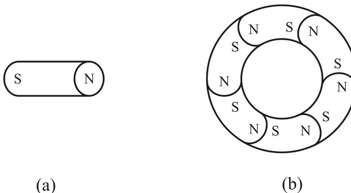
Figure 9.3: (a) Cylindrical magnet. (b) Toroidal magnet.
