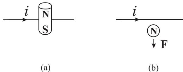
Figure 3.5: (a) Simplified representation of figure 3.4, seen sideways. (b) The experiment seen from above. The letter  $F$  represents the force exerted by the horizontal wire on the vertical needle.
