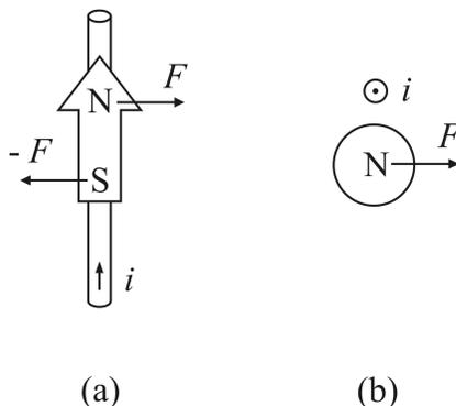
Figure 16.1: (a) Forces exerted by a long and straight current-carrying wire and acting on the supposed magnetic poles of a compass needle  $NS$  aligned with the wire, according to the conceptions of Ørsted, Biot, Savart and Faraday. (b) A cross section of the previous situation. The current  $i$  of the wire is leaving the paper in this representation and we see only the upper North pole of the magnet.
