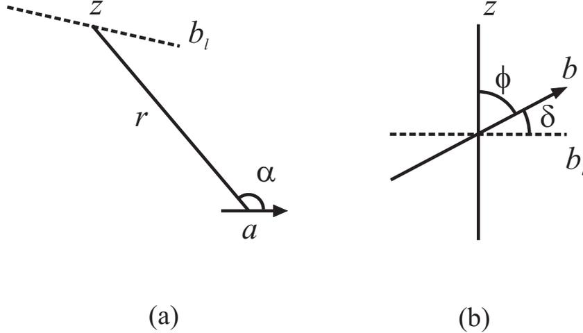
Figure 14.2: (a) Plane  $xy$  formed by the infinitesimal length  $ds$  of the current element  $a = ids$  and by the segment  $r$ . (b) Plane formed by the  $z$  axis, by the length  $ds'$  of the current element  $b = i'ds'$  and by the projection  $b_l$  of the current element  $b$  on the  $xy$  plane.
