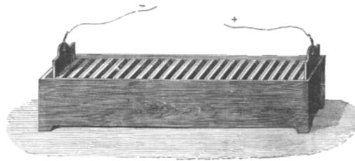
Figure 2.8: Trough battery.
