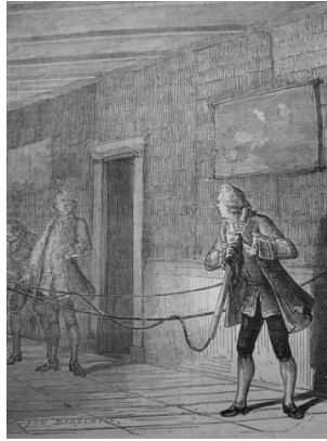
Figure B.9: Gray rubs his 1 m long flint glass tube with his bare hands. A packthread connected to the tube is supported by a silk thread. An ivory ball connected to the other end of the packthread attracts brass leaf beneath it.
