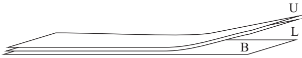
Figure 5.10: The U tape lies on top of the L tape, which lies on top of the B tape.
