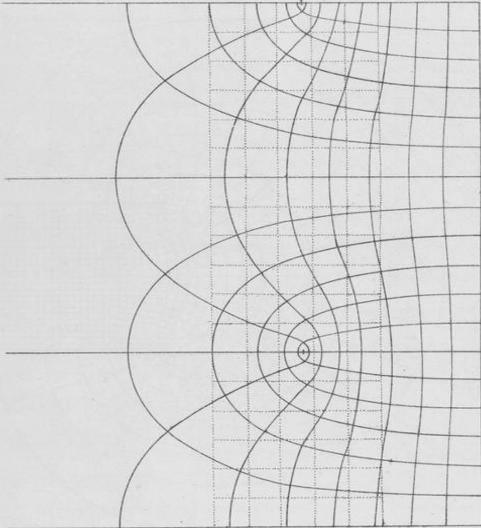
*Lines of Force near the edge of a Plate.*
