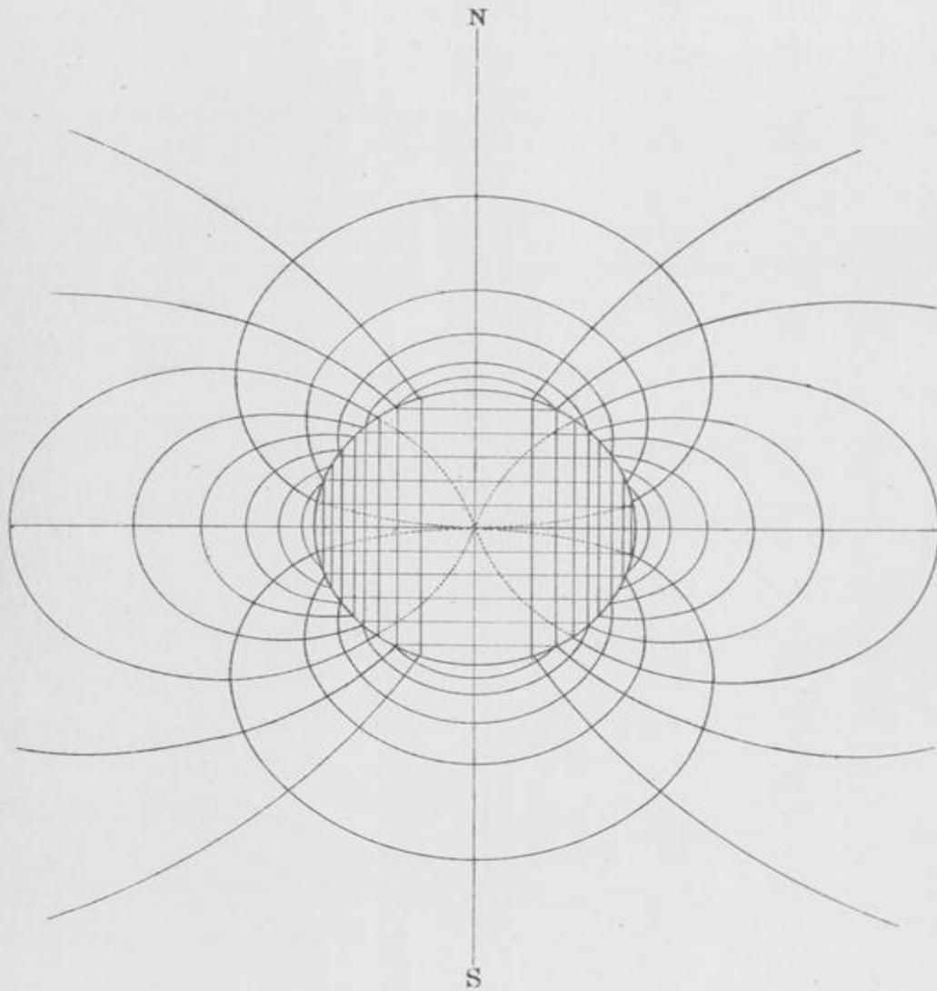
*Lines of Force and Equipotential Surfaces in a diametral section of a spherical Surface in which the superficial density is a harmonic of the first degree.*
