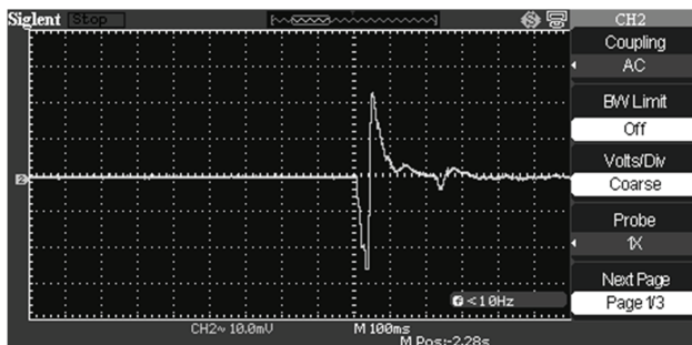
Fig. 51. Pulse, obtained with the break of wire
