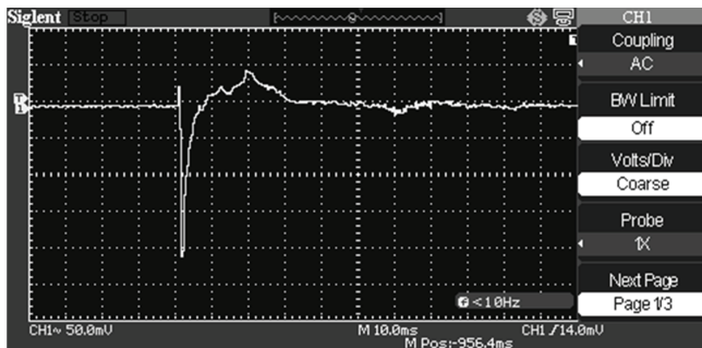
Fig. 46. Shape of pulse after a drop in the rod on the bottom of internal capacity
